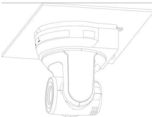
3. Then remove the screws on the hanger and the machine
