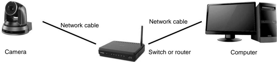
2. To connect directly through network cable, the IP address of the computer should be changed so that it is on the same network segment as the camera
